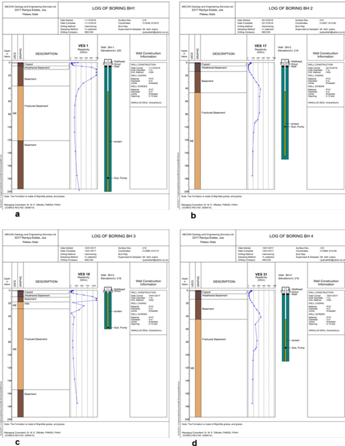
**Fig. 5:** VES-Borehole correlation (Source: Mecon Geology and Engineering Services Ltd.)
