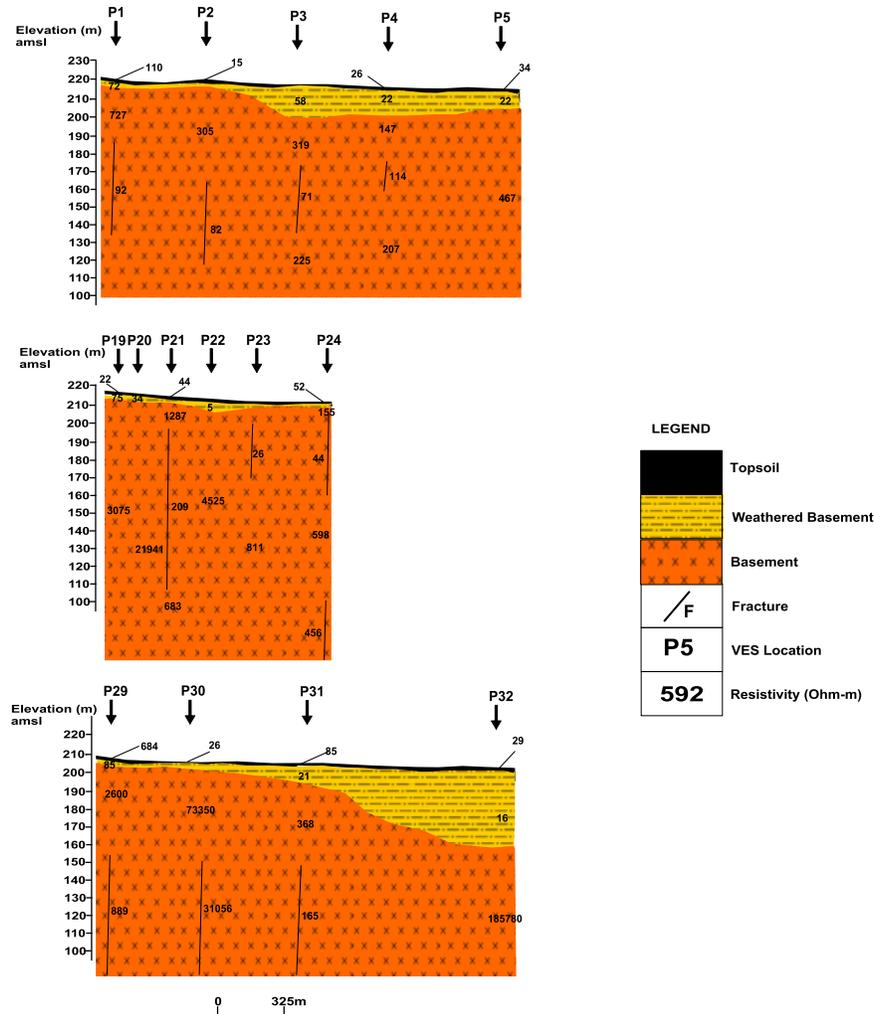
**Fig.4:** Geo-electric section in W-E and N-S directions.
